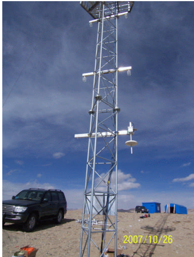
Figure 10. The 40m weather tower with CT2 sensors and temperature sensors at 36.65m, 19.15m, 10.15m, 6.25m, and 4.15m, and the barometer at 2.65m. (Left) The lowest stay hangs the barometer and other two keep a pair of CT2 sensors and a temperature sensor.
