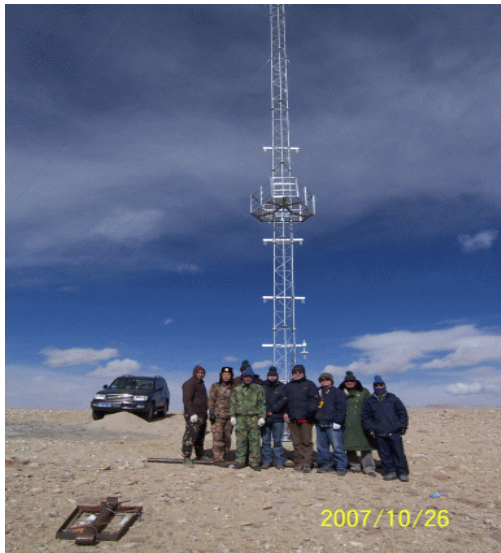
Figure 10. The 40m weather tower with CT2 sensors and temperature sensors at 36.65m, 19.15m, 10.15m, 6.25m, and 4.15m, and the barometer at 2.65m. (Left) The lowest stay hangs the barometer and other two keep a pair of CT2 sensors and a temperature sensor.
