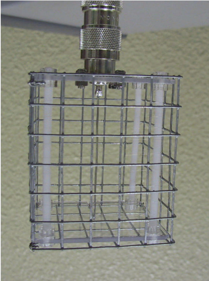
Figure 3. CT2 sensor spiral-bound with a thin nickel wire of 25.4\ \mu\text{m} thick and about 1.9 m long. Resistance is kept about 270\ \Omega within \pm 3.0\ \Omega . The mesh guard is for protecting the nickel wire. Base plates are made of acrylic resin and four supporting rods of Delrin.
