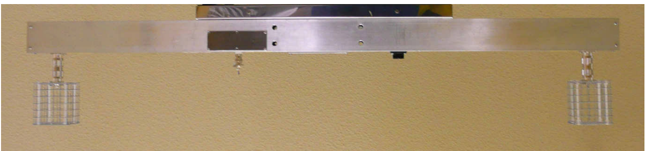
Figure 4. A pair of CT2 sensors are attached to a support stay at left and right end. The separation is 1 m apart. A temperature IC sensor, AD590MH (Analog Devices), is installed close to the center of the stay.
