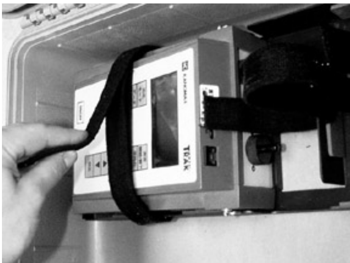
Figure B-9: Tighten the Velcro Strap
