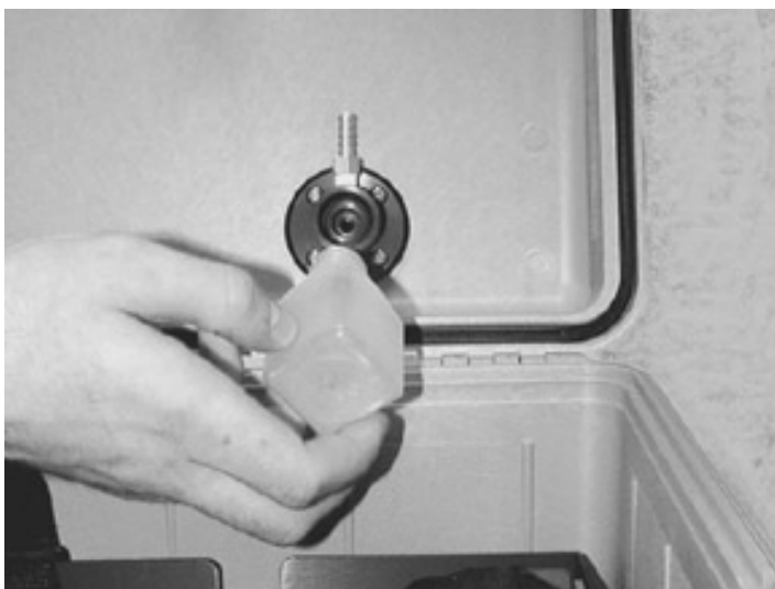
Figure B-5: Installing the Water Trap Bottle
