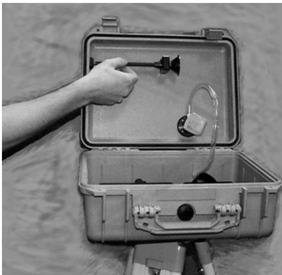
Figure B-3: Unscrew Inlet from Inner Bracket
