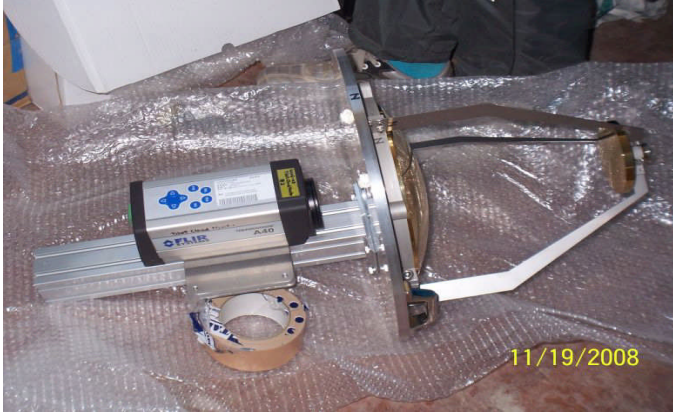
④ M1 base-plate with M2 spiders, MIR camera
