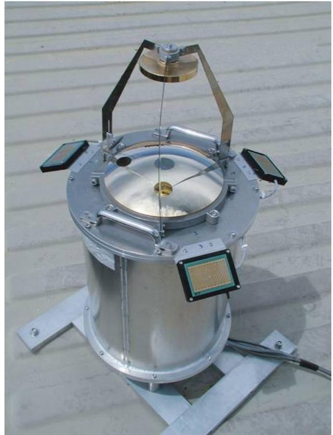
FIG. 2.—Outdoor part of the MAGNUM infrared cloud monitor. Shown from top to bottom are the secondary mirror, primary mirror, and aluminum pipe housing that contains the thermal imager, signal converter, shutter controller, etc. The three rectangular plates extending from the upper edge of the housing are rain sensors that form a different system from the cloud monitor but share power and wiring.
