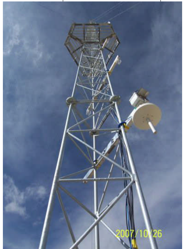
CT2 sensors and a barometer at Karasu
