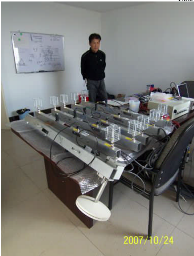
Five sensor base rods for CT2 sensors and a barometer, and its controller at Kashi
