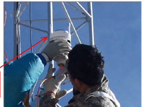
④ a weather monitor on the tower
