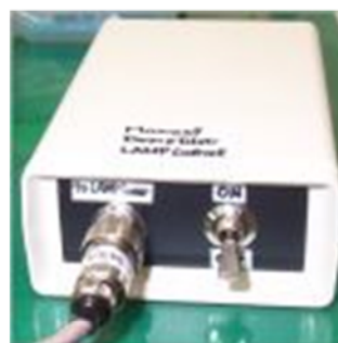
Fig.1-3 A remote control box for Dome-Flat illumination lamps, operated manually.
