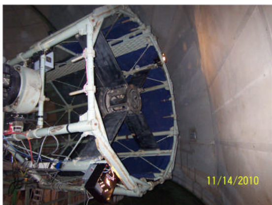
Fig. 1-1 Two Dome-Flat lamps, installed both sides of the tube top of Kottamia 188 cm telescope, which are illuminating the wall inside the dome.
