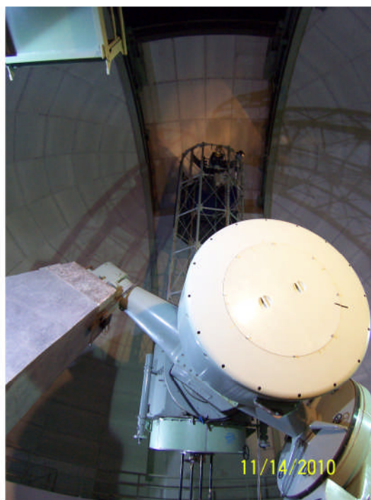
Fig. 1-2 Dome-Flat lamps are illuminating the dome slit when the telescope near the zenith. Shadows are of telescope structures lighting by interior lamps around the dome.
