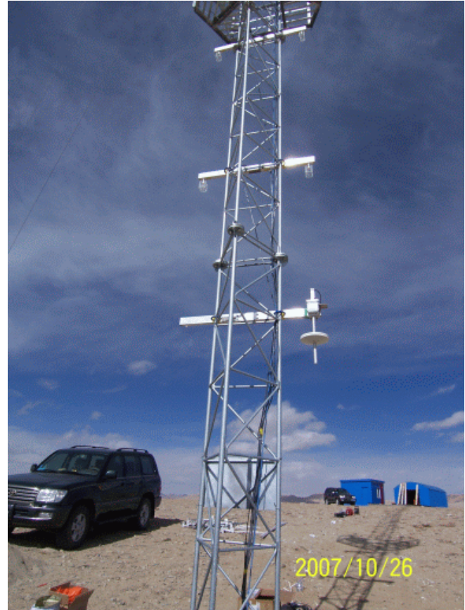
Figure 10. The 40m weather tower with CT2 sensors and temperature sensors at 36.15m, 19.15m, 10.15m, 6.25m, and 4.15m, and the barometer at 2.65m. (Left) The lowest stay hangs the barometer and other two keep a pair of CT2 sensors and a temperature sensor.
