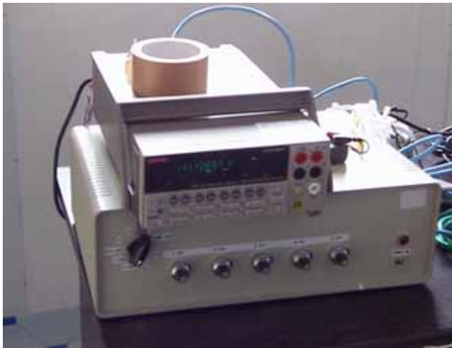
Figure 8. A control box (below) contains the circuit board for CT2. Above the control box is a data acquisition system, KEITHLEY Integra 2701 with I/O card 7702, which digitize voltages and transfer them to PC via Ethernet connection.
