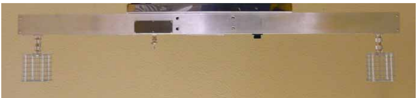
Figure 4. A pair of CT2 sensors are attached to a support stay at left and right end. The separation is 1\ \text{m} apart. A temperature IC sensor, AD590MH (Analog Devices), is installed close to the center of the stay.
