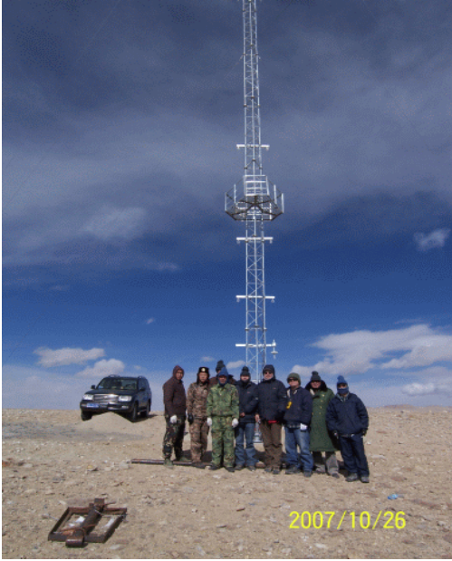
Figure 10. The 40m weather tower with CT2 sensors and temperature sensors at 36.15m, 19.15m, 10.15m, 6.25m, and 4.15m, and the barometer at 2.65m. (Left) The lowest stay hangs the barometer and other two keep a pair of CT2 sensors and a temperature sensor.
