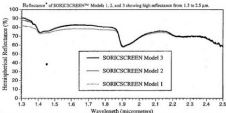
\* Reflectance measurements shown represent the minimum reflectance since a black backing plate was used. Actual reflectance during use may be higher for non-black backgrounds. Reflectance measurements are 8° hemispherical reflectance (traceable to NRCC - the National Research Council of Canada) measured on a 150 mm diameter Labsphere RSA-PE-19 integrating sphere accessory on a Perkin Elmer Lambda 19 Spectrophotometer.
