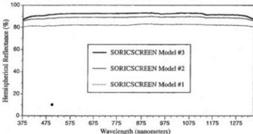
\* Reflectance measurements shown represent the minimum reflectance since a black backing plate was used. Actual reflectance during use may be higher for non-black backgrounds. Reflectance measurements are 8° hemispherical reflectance (traceable to NRCC - the National Research Council of Canada) measured on a 150 mm diameter Labsphere RSA-PE-19 integrating sphere accessory on a Perkin Elmer Lambda 19 Spectrophotometer.
